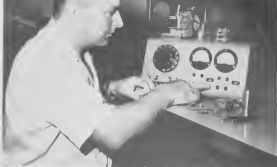
MAX SAND, technical assistant in the Instrument Shop, adjusts a control on the testing device he invented and designed for testing components for the lab's Automatic Standard Distillation Apparatus. For his
